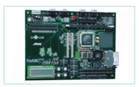
The SDB-750/1000 is powered by the ARM7TDMI 32-bit RISC processor based AT91R40807. In combination with the 2 Mbytes SRAM and 16 MBytes of program memory (FLASH), the board operates in a standalone mode. It is available with an up to one million gates ProASIC PLUS FPGA from Actel.
